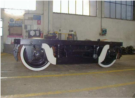
Construction of new bogies for Orient Express
